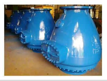
Recoil of a gun - soon as the bullet is fired, the gunner (at least the firing arm) is thrown back in recoil almost instantaneously. Pretty much in the same way, as soon as the pump trips, the door proceeds to close, the last bit of travel slowed down due to the large girth (and therefore voluminous cavity) around the seat and the door closes finally without slamming. No external dampening or counter weight used.
