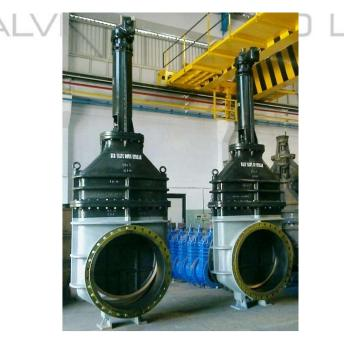
The valve was manufactured complying fully with the specs given by client, inspected thoroughly (stage wise by IHI engineers) and supplied. Both the valves fixed into a short pipeline and then concrete poured leaving half the valve buried within with only a tiny chamber kept on top for the operator to come in and operate the valve.
