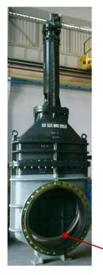
The extent to which the rising stem projects above the valve is a visual indicator of the extent of its opening. Thus the operator is spared the trouble of going near the valves to check if it is open or closed.
